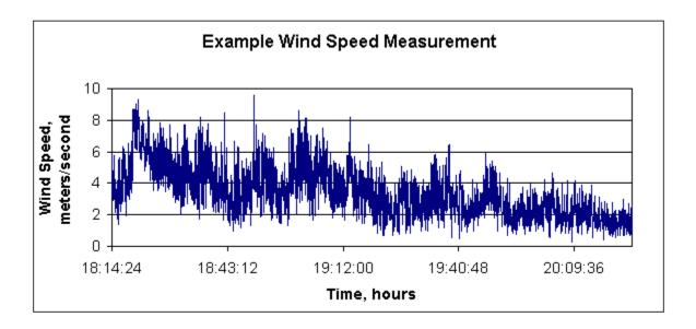
The graphs show considerable fluctuations of wind speed and direction with time. The third graph is a 15-minute blowup of a section of the second graph which expands 3 hours.
