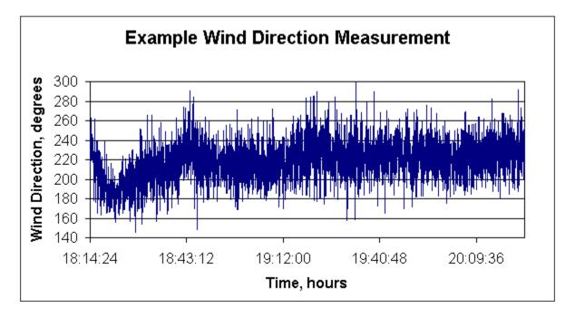
For the example presented, the wind sensor was placed two meters above the ground. The time represents hours since midnight (standard time) on August 28, 1995. Data was recorded at one-second intervals
